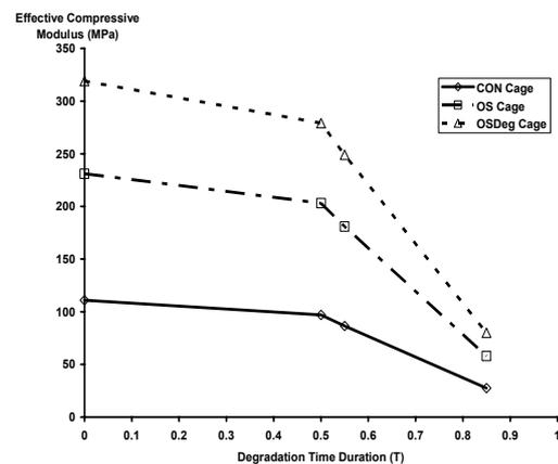
Figure 5: The comparison of effective compressive moduli of PPF/β-TCP cages of CON, OS, and OSDeg designs through the degradation.
