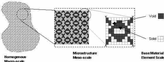
Figure 1. Schematic processes show the homogenization method to design the topology optimized microstructure that achieved the desired effective material properties.
