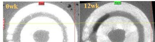
Figure 4: The comparison of the image density of the PPF/β-TCP CON cage design taken from micro-CT scan. The images showed a decayed intensity of the grayscale level without geometrical change, indicating an undergoing bulk erosion mechanism from 0 week to 12 weeks.
