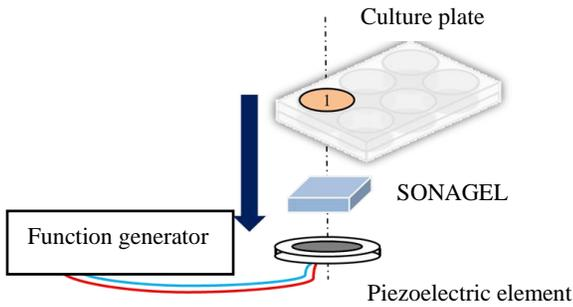
**Fig. 2:** How to apply vibration.
