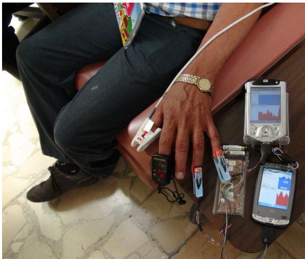
Fig. 15. Oximeters test; Mazimo, Nonin and Oximeter WiFi in a patient.
