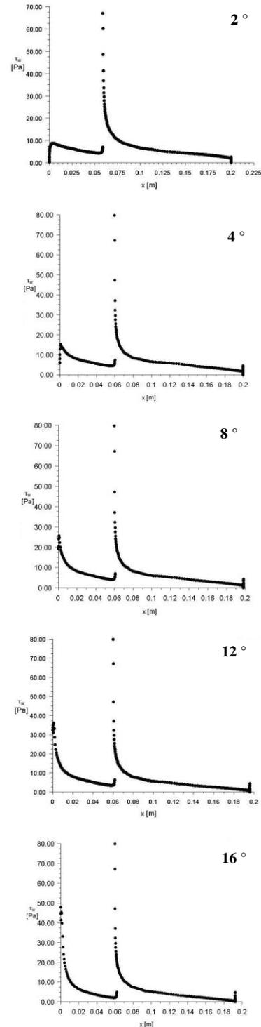
Figure 16. Wall shear stress of the 2415-3S airfoil at blowing condition for different AOA.
