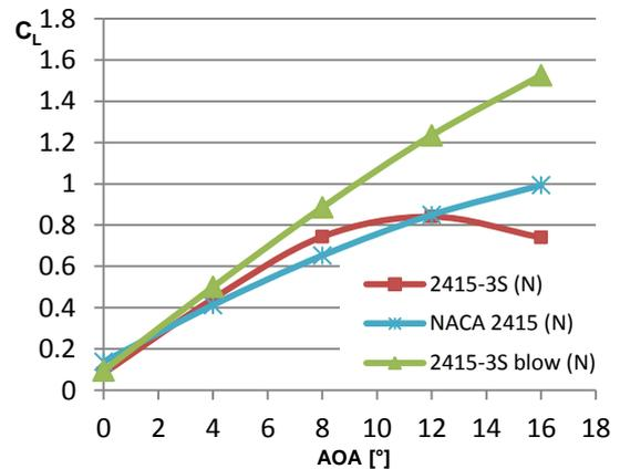
Figure 12. Numerical lift coefficient for 2415-3S airfoil for blowing and gliding conditions and NACA 2415 airfoil.
