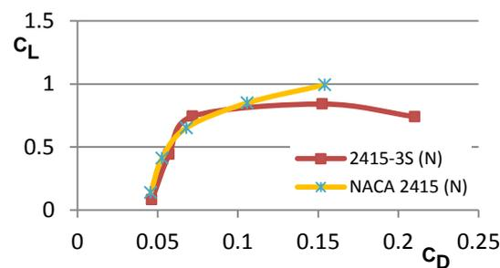
Figure 7. Numerical polar graph for 2415-3S and NACA 2415 airfoils.
