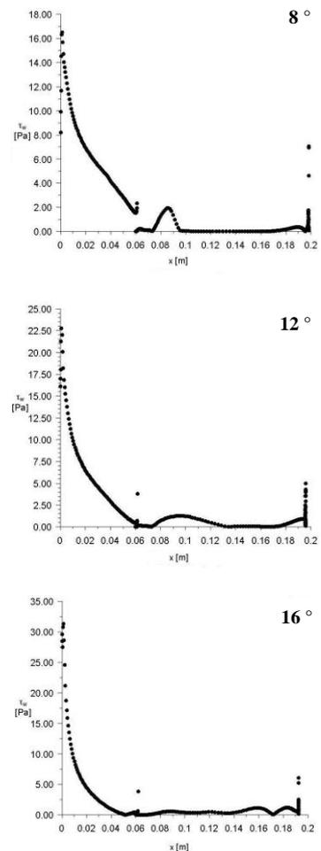
Figure 9. Wall shear stress of the 2415-3S airfoil at gliding condition for different AOA.
