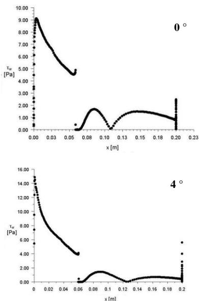
Figure 9. Wall shear stress of the 2415-3S airfoil at gliding condition for different AOA.
