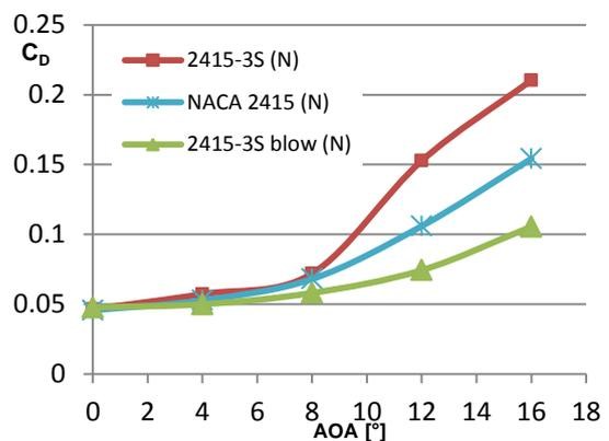
Figure 13. Numerical drag coefficient for 2415-3S airfoil for blowing and gliding conditions and NACA 2415 airfoil.
