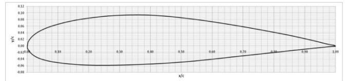
Figure 2. NACA 2415 airfoil.
