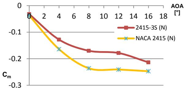
Figure 8. Numerical pitching moment coefficient for 2415-3S and NACA 2415 airfoils.
