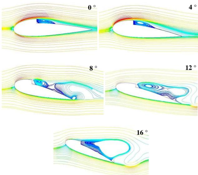
Figure 11. Streamlines of the 2415-3S airfoil at gliding condition for different AOA.
