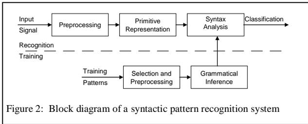
Figure 2: Block diagram of a syntactic pattern recognition system
