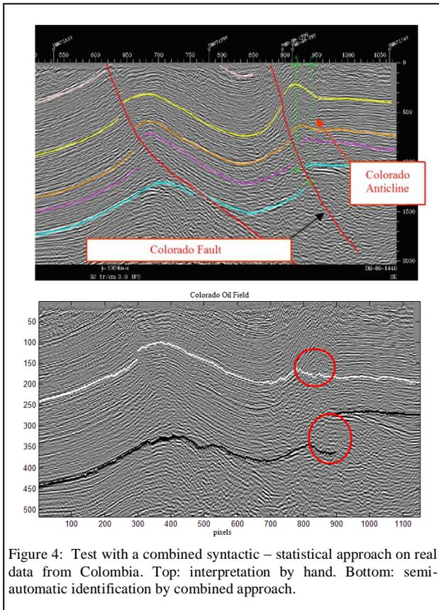
Figure 4: Test with a combined syntactic – statistical approach on real data from Colombia. Top: interpretation by hand. Bottom: semi-automatic identification by combined approach.
