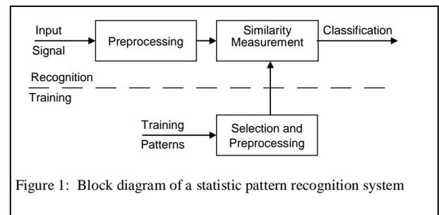
Figure 1: Block diagram of a statistic pattern recognition system
