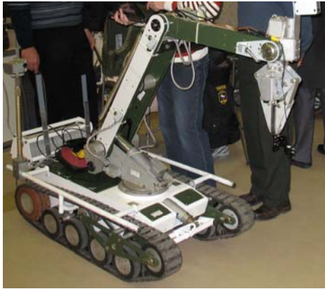
Fig. 2. The registering block of the contactless odometer is mounted in a MRK-27 grasping unit. On fig.3 the example of the displacement vectors detection for concrete floor scenes is shown. Frequency of the displacement vectors generation not less than 10 Hz.
