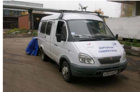
Fig. 10. The general view of Mobile Laboratory for Operative Diagnostics of a road surface (MLOD).
