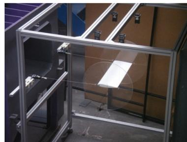
Figure 2. Location of scales in the aerodynamic balance.
