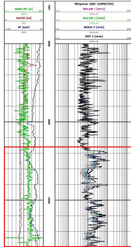
Fig. 4: Array laterolog resistivity curves logged in the upper and middle Bossier formation. Note the resistivity curve separations in the middle Bossier log response (boxed in red).
