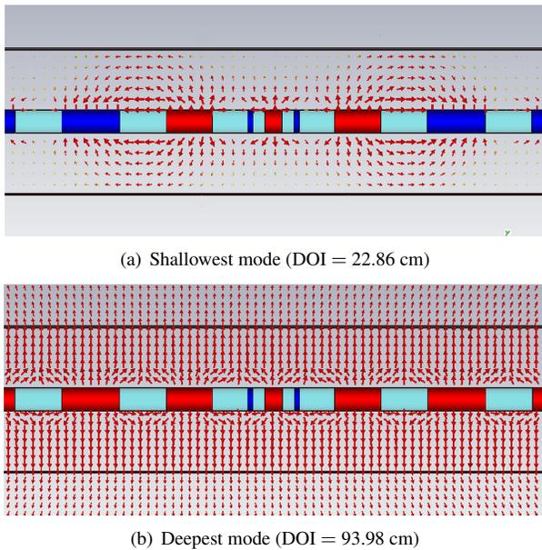
Fig. 7: Current density maps in  $y$ - $z$  plane for array laterolog in formation with vertical resistive fractures
