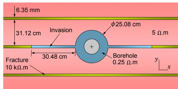
Fig. 5: 3-D model with vertical resistive fractures proposed to explain resistivity curve separations
