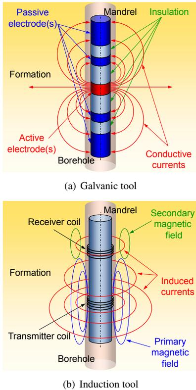
Fig. 1: Schematic diagrams of two typical kinds of resistivity tools
