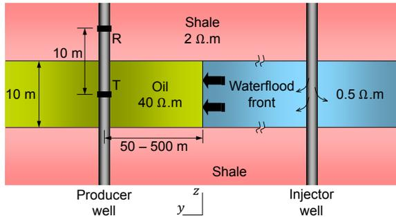
Fig. 10: 3-D model to study the feasibility of reservoir monitoring using TEM borehole technology
