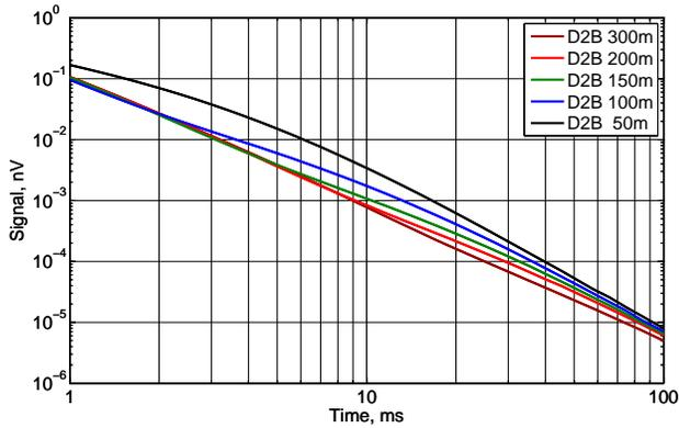
Fig. 9: Simulated coaxial receiver signals as a function of time for different distances (D2B) between the waterflood front and the producer well
