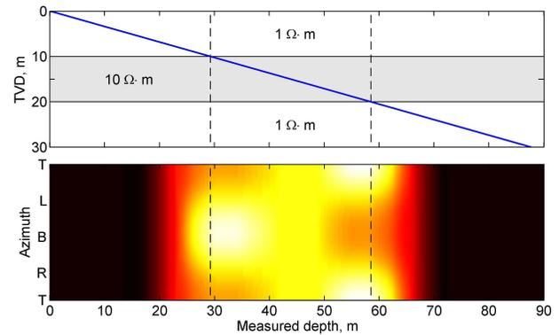
Fig. 2: Simulated deep resistivity image for a straight-line well trajectory entering and leaving a reservoir at 70° relative dip
