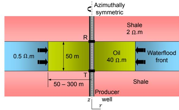
Fig. 8: Proof-of-concept model for reservoir monitoring using TEM borehole technology
