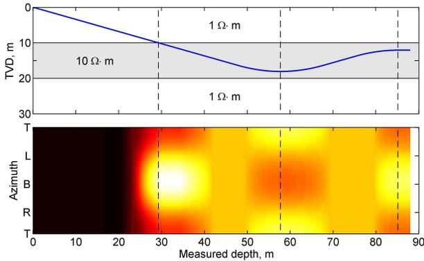
Fig. 3: Simulated deep resistivity image for a realistic geosteering scenario where the well is landed in the reservoir at 70° relative dip and then steered to stay within the reservoir close to the roof
