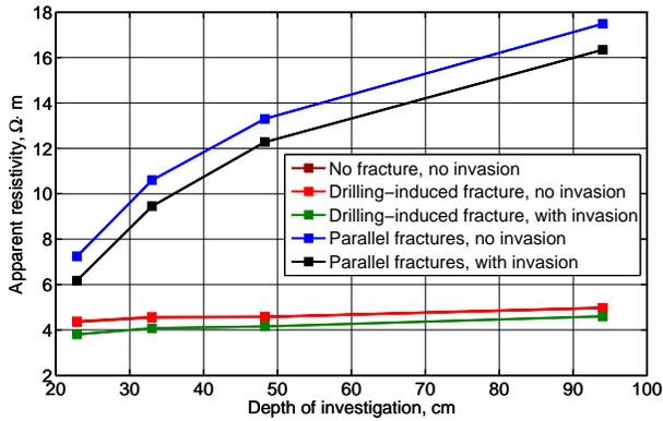
Fig. 6: Simulated array laterolog apparent resistivity as a function of DOI for different fracture and invasion cases
