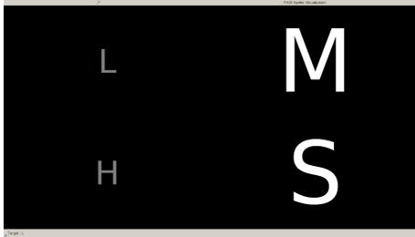
Fig. 3: P300 visualization is divided into four states: Low-speed, Medium-speed, High-speed and Stop. A fifth state is detected by the system when the user is not looking at the screen.
