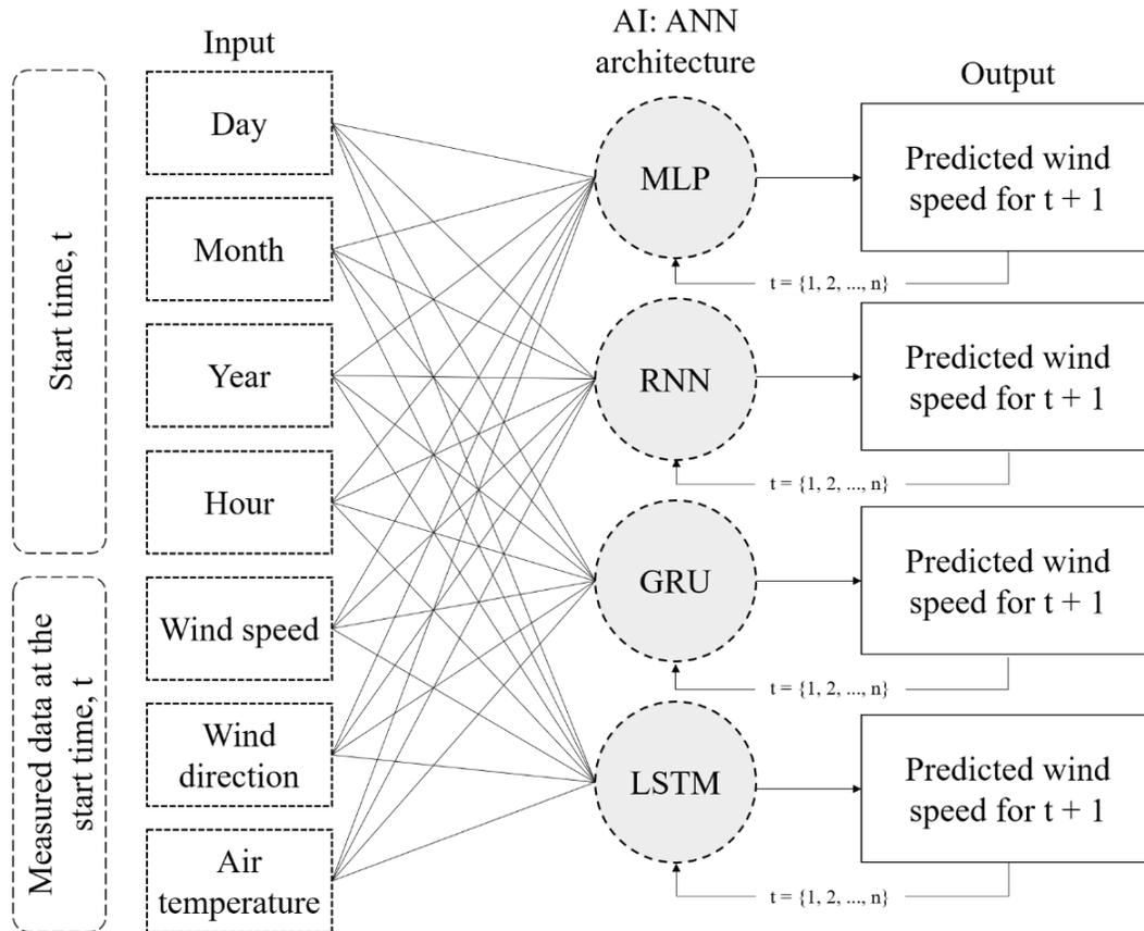
**Figure 5:** Workflow of the supervised machine learning AI wind speed forecasting procedure for 1 h to 12 h ahead of the start time.
