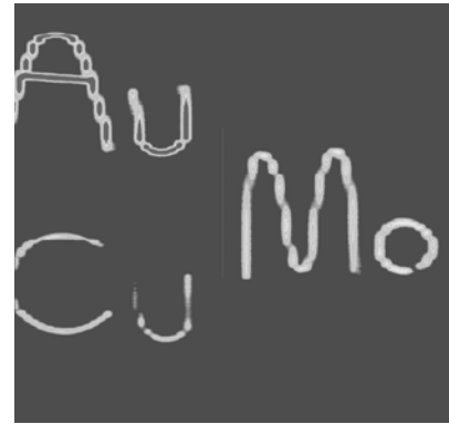
Fig. 3 Material discriminated X-ray penetration image of copper (Cu), Molybdenum (Mo), and Gold (Au).
