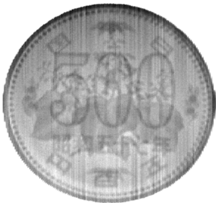
Fig. 2 X-ray penetration image of 500-yen coin.
