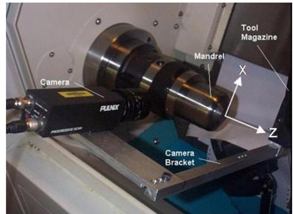
Figure 4: Tool magazine mounted camera
