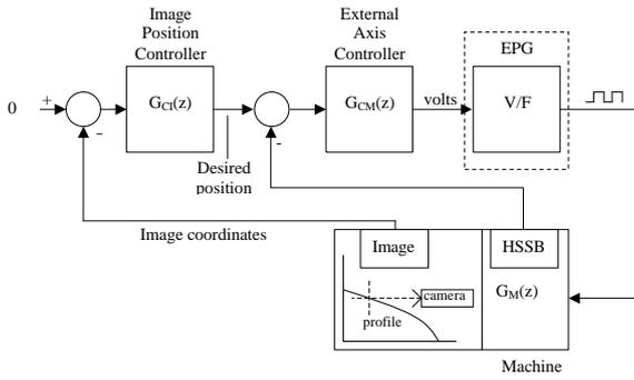
Figure 3: The active axis control system
