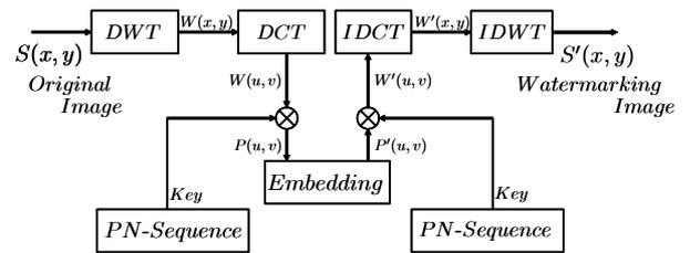
Fig. 2 Embedding Watermarking System
