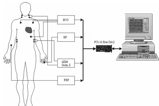
Figure 1. Configuration used for the virtual instrument.
