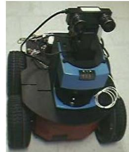
**Fig. 2.** Pioneer 3-AT outdoor mobile robot.
