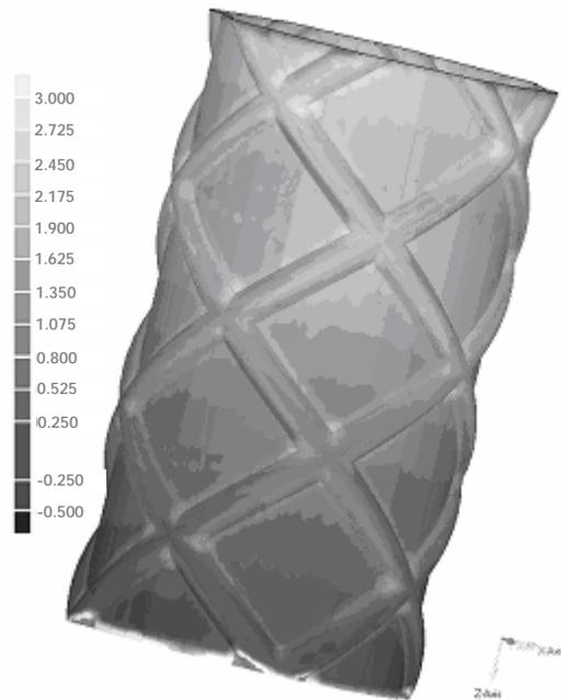
Figure 8 3D scanned data registered to CAD STL model
