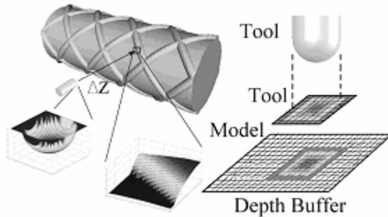
Figure 4 Depth buffer tool positioning
