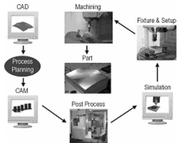
Figure 1 CNC machining process (reproduced from Gray et. al. [1])
