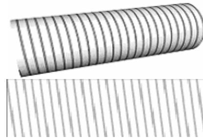
Figure 3 Helical tool path
