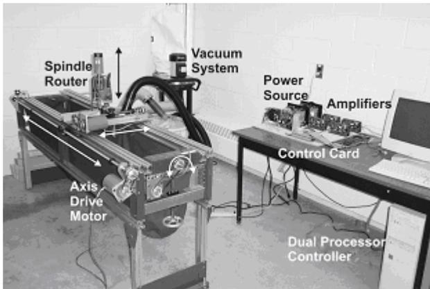
Figure 9 4-Axis Router machine
