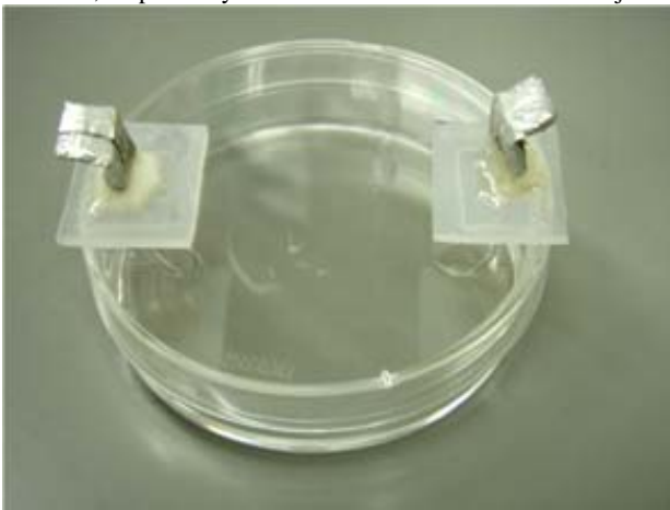
Fig. 3: A pair of electrodes attached on the cover of the culture dish.
