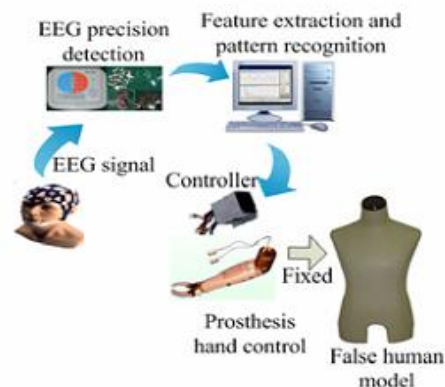
Fig.1 The neural prosthesis hand system driven by BCI
