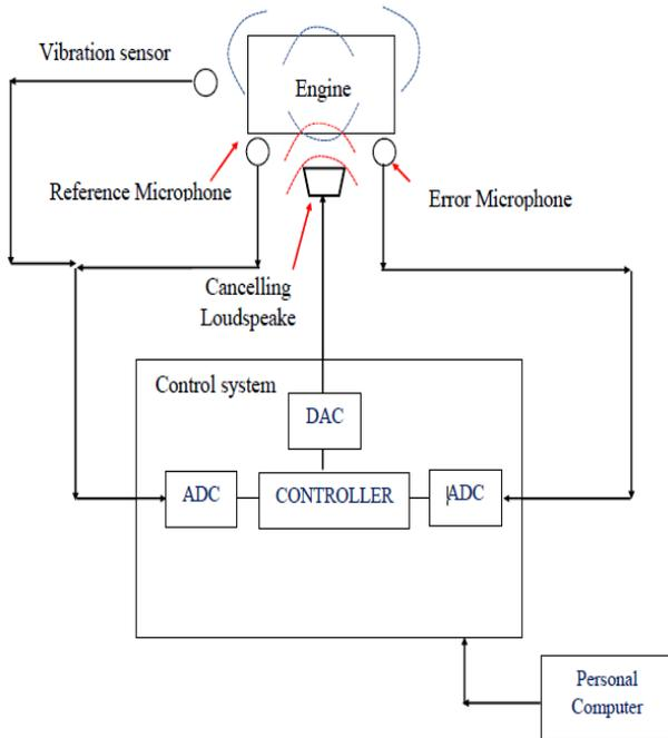
Figure 5. Setup configuration.
