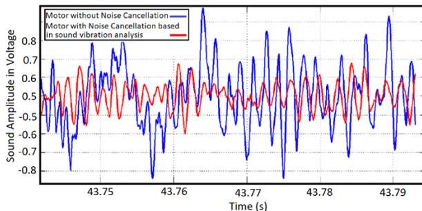
Figure 6. Experimental test in time domain for a DC motor joined to an Active Magnetic Bearing System.
