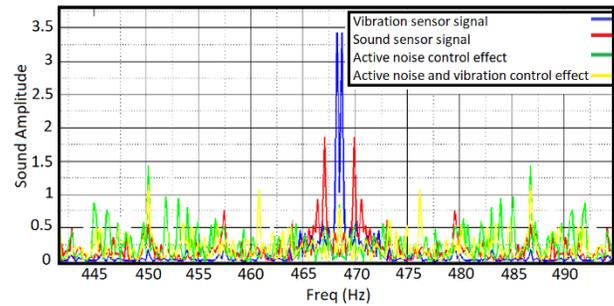
Figure 7. Frequency domain experimental comparisons.
