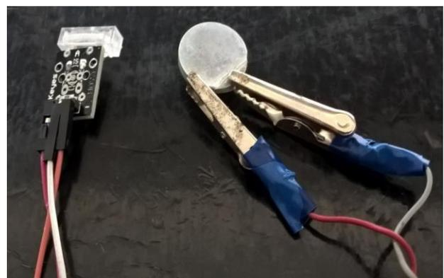
Figure 2. Vibrations sensors
