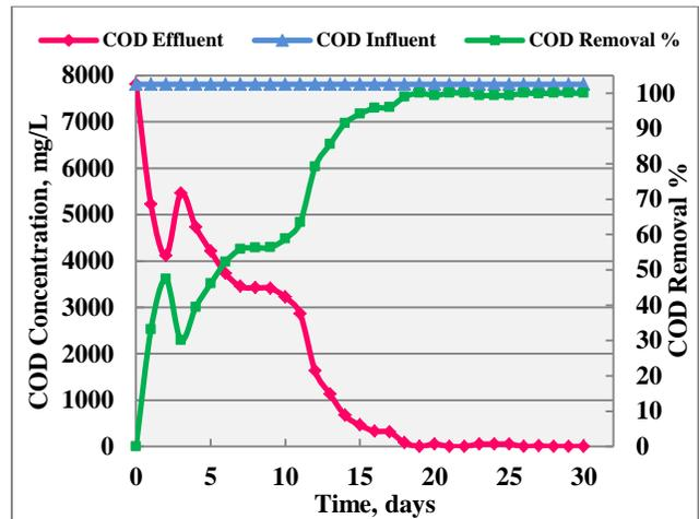
Fig.4 Profile COD removal in membrane less-MFC
