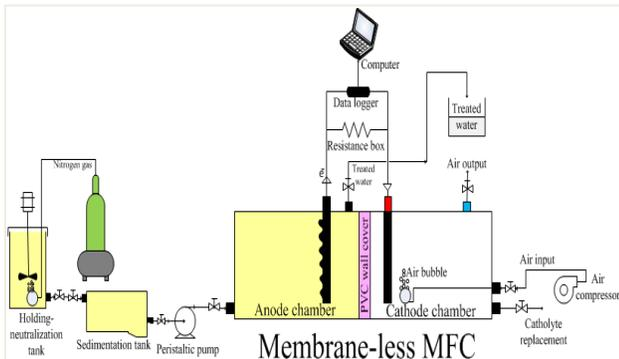
Fig. 3 membrane-less complete system
