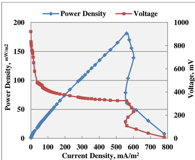
Fig. 6 Polarization curve for membrane-less MFC
