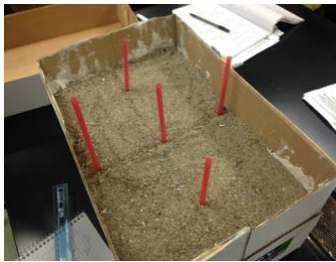
Figure 1b. Box with the sand added and five straws used to estimate the volume of sand in the box.
