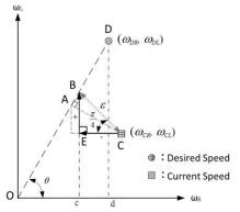
Fig. 5. The traditional and the proposed cross-coupling control methods.
