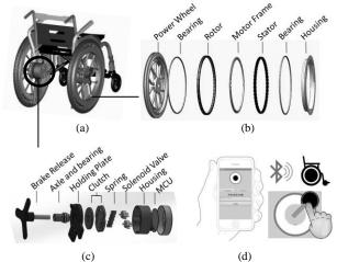
Fig. 2. (a) Configuration of the smart wheelchair driven by dual power wheels, (b) rim motor in the power wheel and its components, (c) brake assembly, and (d) remote control on the smart phone.
