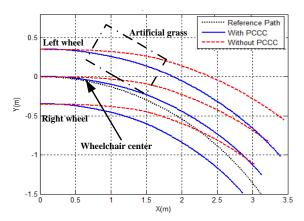
Fig. 7. Trajectories of the left and right wheels before and after the wheelchair drives through the artificial grass with and without the proposed cross-coupling control.
