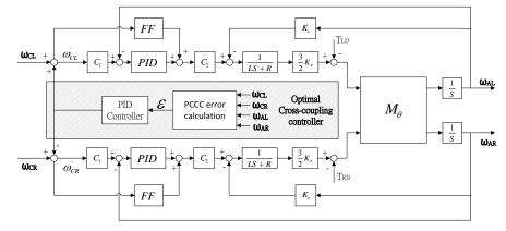
Fig. 4. Optimal cross-coupling control structure.
