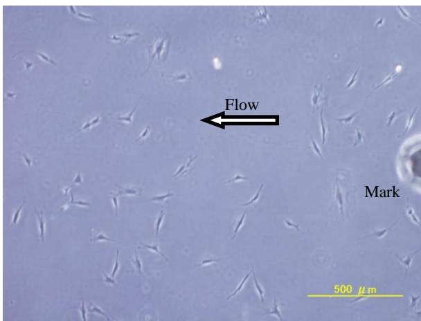
Fig. 6b: MC3T3-E1 just after shear flow simulation (1.9 Pa) for 30 minutes. Dimension from left to right is 2 mm.
