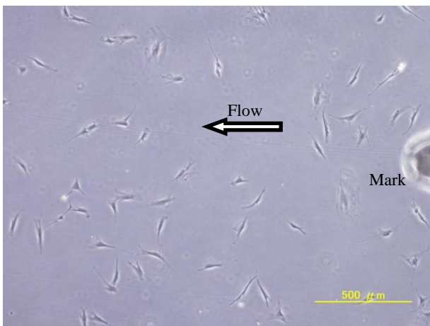
Fig. 6c: MC3T3-E1 at 30 minutes after shear flow simulation (1.9 Pa). Dimension from left to right is 2 mm.
