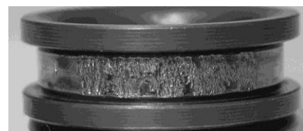
Fig. 3: Spalled inner ring raceway of the tested cylindrical roller bearing.
