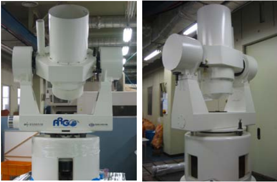
Figure 10. Manufactured prototype of ARGO-M tracking mount
