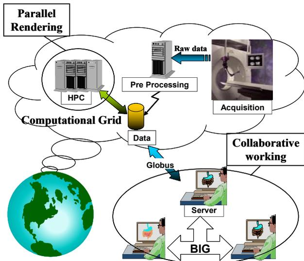
**Fig. 2.** Use of Computational Grids to build a collaborative environment for biomedical imaging.
