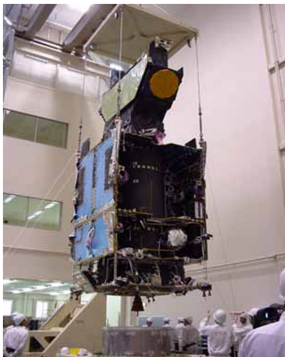
Figure 3. ETS-8 Flight Model Integration (Summer 2003)
