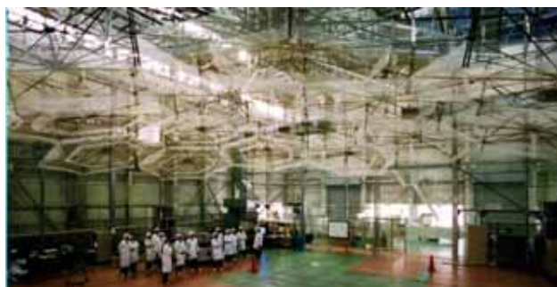
Figure 4. ETS-8 LDR Deployment Ground Test
