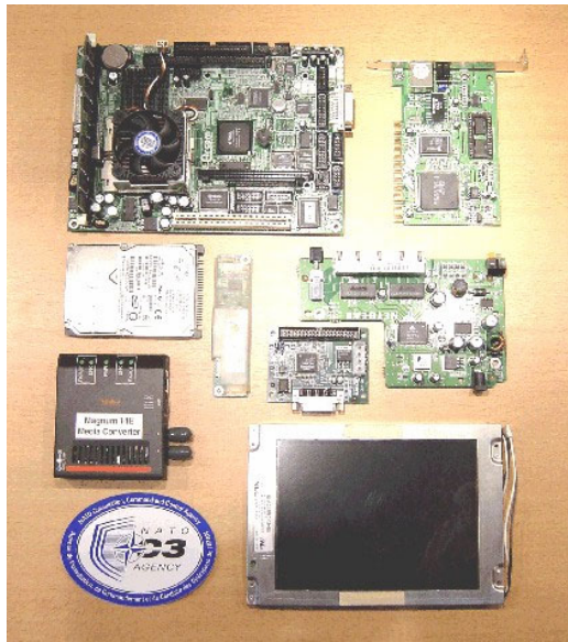
Figure 6. Typical parts in a Remote Monitoring Device (RMD)
