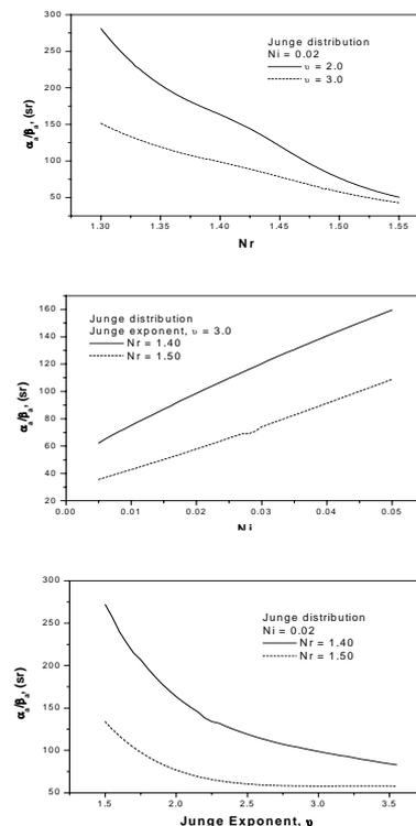
Fig. 1 Variation of  $S_1$  with  $N_r$ ,  $N_i$ , and  $v$
