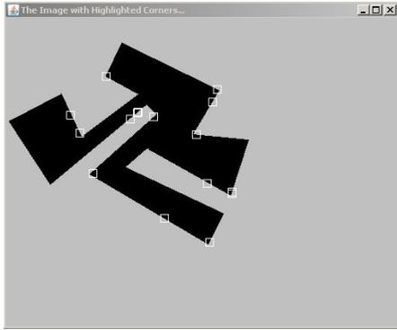
Fig 3. An example test image where the Moravec operator has identified high interest corner points.
