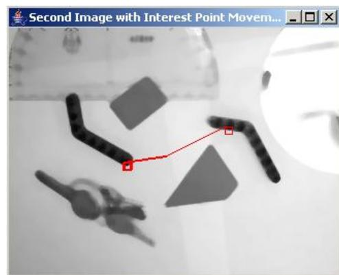
Fig. 6 Example screenshot at the eleventh iteration of the algorithm which contains an incorrect interest point correspondence.
