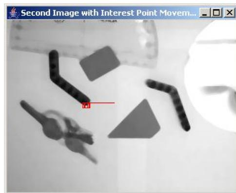
Fig. 7 Example screenshot at the twenty third iteration of the algorithm which shows perfect horizontal movement of the interest points which causes the algorithm to terminate.
