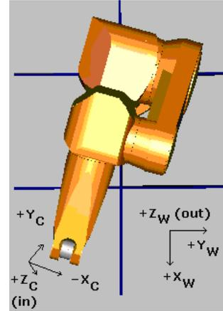
Fig 2. An example initial alignment of camera and robot frames. The unknown angle differences are recovered by the algorithms in the following sections.
