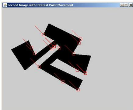
Fig 4. A second example test image in which the camera has moved and the correspondences and movements of the interest points are drawn on top it.
