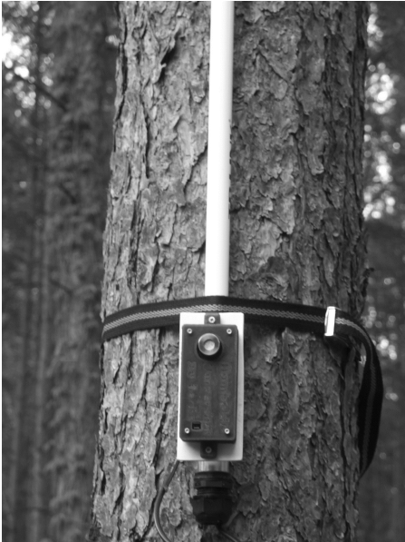
Figure 4b: Forest fire sensor with antenna on a Scots pine tree.
