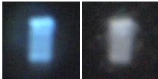
Figure 12: Further comparison of CWO (left) and BGO (right) scintillators at a photon energy of 12.6613 keV and temperature of 100 K. The field of view is 170 x 170 μm 2 .
