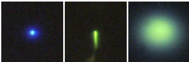
Figure 5: The X-ray penetration into CWO (left), YAG:Ce (center), and Gd 2 O 2 S:Tb phosphor (right) excited by the 12
