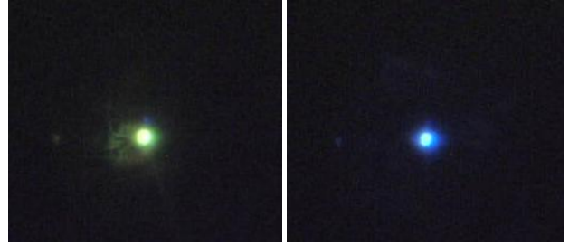
Figure 6: On-axis view of the 5 μm x-ray minibeam, using YAG:Ce (left), and CWO (right). The beam intentionally is saturating the camera pixels. Each image is about 340 x 300 μm 2 .
