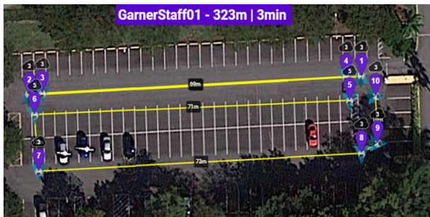
Figure 2: Flight automation of a parking lot.
