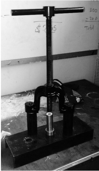
Figure 4. Screw press built to make the pellets.
