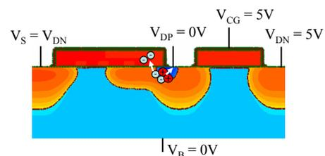
Fig. 4 : Erasing of the new single-poly cell double implant by a Zener effect
