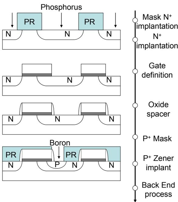
Fig. 2 : Process flow of the new single-poly cell double implant
