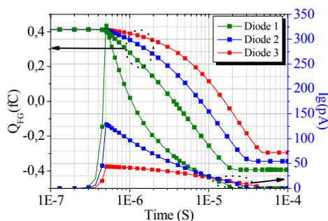
Fig. 9 : Cell erasing Qfg(time) and Ig(time) for the different diodes implantations
