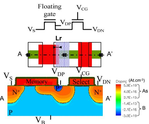
Fig. 1: (a) Layout, (b) schematic and (c) cross section of a TCAD process simulation of the new single-poly cell double implant
