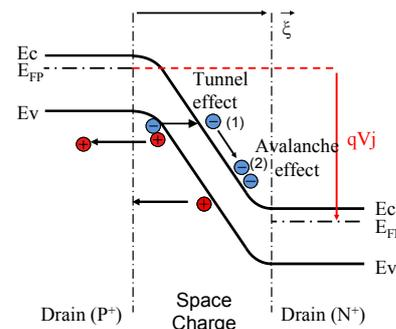
Fig. 3 : Tunnel and avalanche effect on a diode
