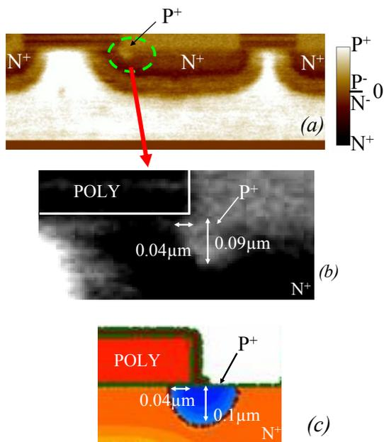
Fig. 8 : (a) AFM SCM cut and (b) zoom on the poly-silicon overlap of the P<sup>+</sup> implant (c) TCAD process simulation of the double implant
