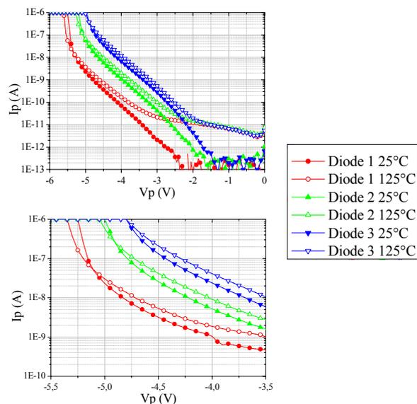
Fig. 7 : (a) Electrical characterizations of Zener diodes and zoom on breakdown temperature shift at  $1\mu\text{A}$  (b) Zoom on the current curves around the Zener to Avalanche effect transition
