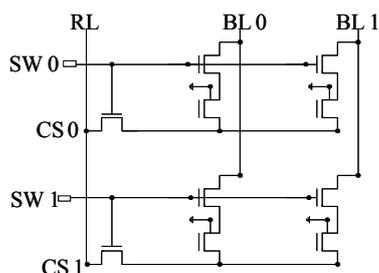
Fig.6 : Array of 4 new single-poly cells double implant
