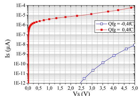
Fig. 11: Cell reading I<sub>S</sub>(V<sub>S</sub>) with |Q<sub>FG</sub>|=0.4fC
