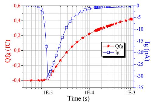
Fig. 10: Cell writing Q<sub>FG</sub>(time) and I<sub>G</sub>(time) for diode 1
