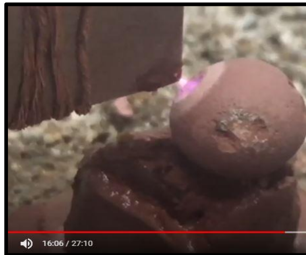
Figure 14: Screenshot of Brown’s experiment demonstrating EDM cratering [23].
