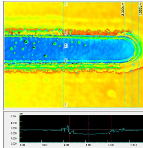
**Fig. 6:** Dimension of groove of mold measured with laser microscope. Lower figure of tracing along vertical direction in upper figure (dimension from left to right is 0.015 mm) shows depth of 0.0007 mm.
