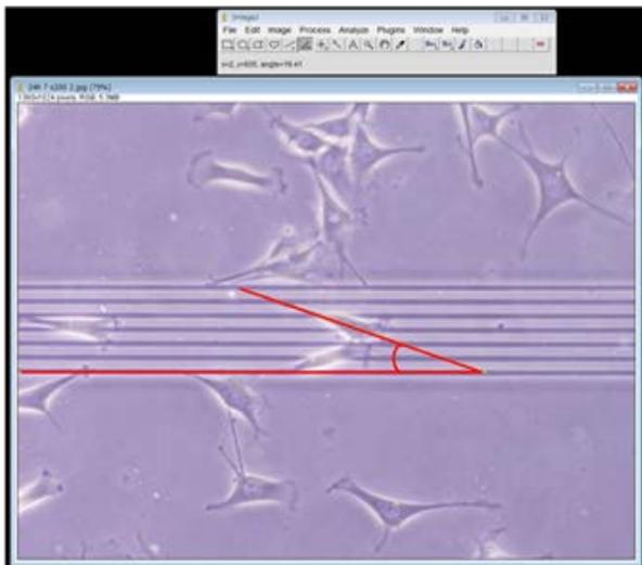
**Fig. 5:** Angle between longitudinal axis of cell and longitudinal direction of ridge. Dimension from left to right is 0.5 mm.
