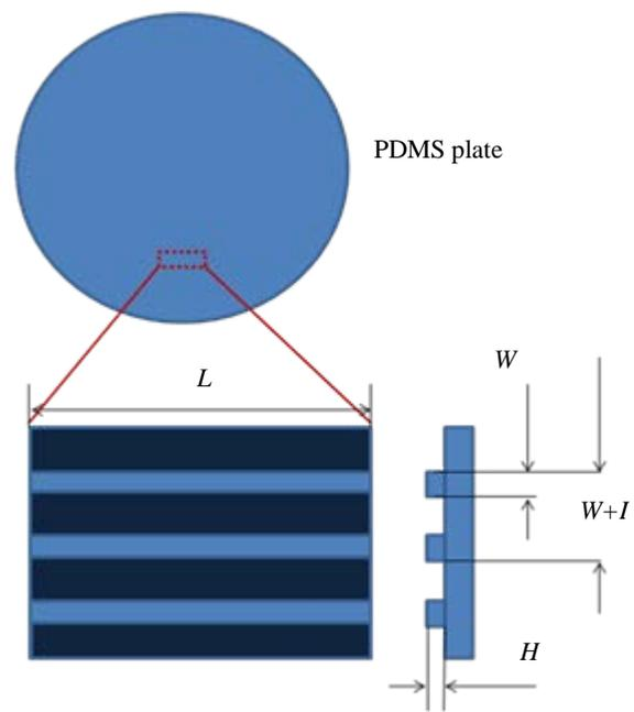
**Fig. 3:** Typical location of micro ridges (magnified in bottom) on the plate of PDMS plate.
