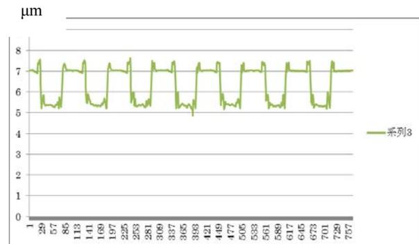
**Fig. 7:** Cyclic gap in tracing of surface of mold with laser microscope shows depth of grooves of 0.0015 mm.
