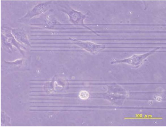
**Fig. 9:** 24 hours of cultivation on ridges of 0.0003 mm height. Cell spreads over the ridges of 0.0003 mm height.
