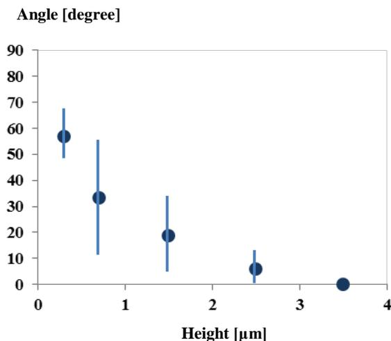
**Fig. 14(B):** Mean angle (point) between longitudinal axis of cell and longitudinal direction of ridge in relation to height of ridge. The vertical bar shows standard deviation.
