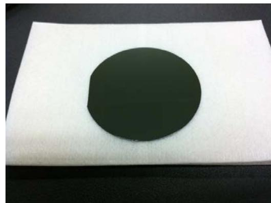
**Fig. 1:** Silicon wafer for mold (diameter: 50 mm).
