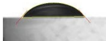
**Fig. 8(A):** Drop of medium on PDMS before oxygen plasma ashing.
