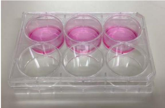
**Fig. 4:** Cell culture on disk of PDMS with micro ridges dipped in the dish of six wells.
