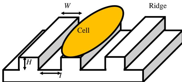
Fig. 15(A): Orientation of cell on low ridge.
