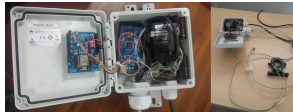
Figure 5: Casing of Outdoor Sensors
