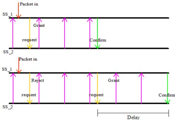
Figure 2: MSH-DSCH interval: SS<sub>1</sub> > SS<sub>2</sub>
