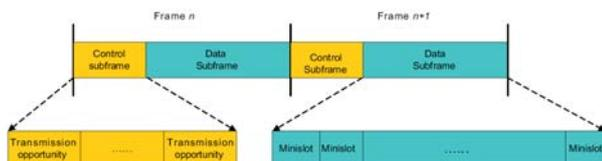
Figure 1: IEEE 802.16 Mesh Frame Structure
