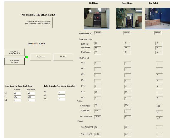
Fig. 5: GUI used by the human operator to obtain sensor feedback, and generate simulated and experimental runs.
