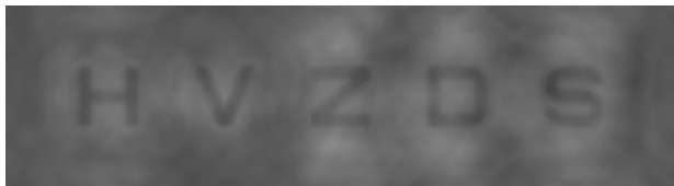
Figure 6- Simulated image of what the subject would see when viewing Figure 3 through the -6.0 diopter lens.
