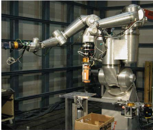
Figure 9. A 17 degree-of-freedom manipulator performing automated tasks.
