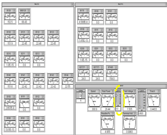
Fig. 12 Raise terminal voltage for Jeju GT#3(0.9 → 1.0pu)
