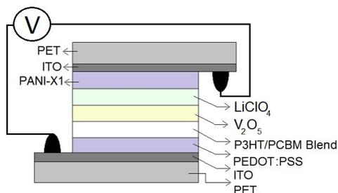
**Figure 1.** Configuration of flexible electrochromic device.
