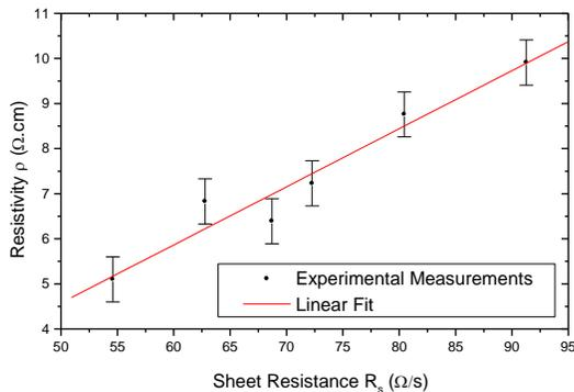
**Figure 3.** Electrical resistivity of the PET/ITO/PANI-X1 in function of sheet resistance.
