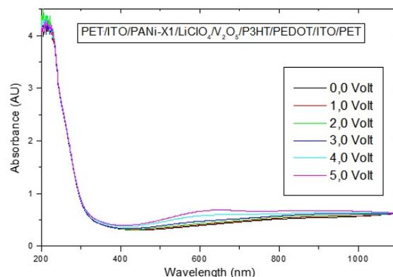
**Figure 2.** UV-Vis spectroscopy of flexible electrochromic device.
