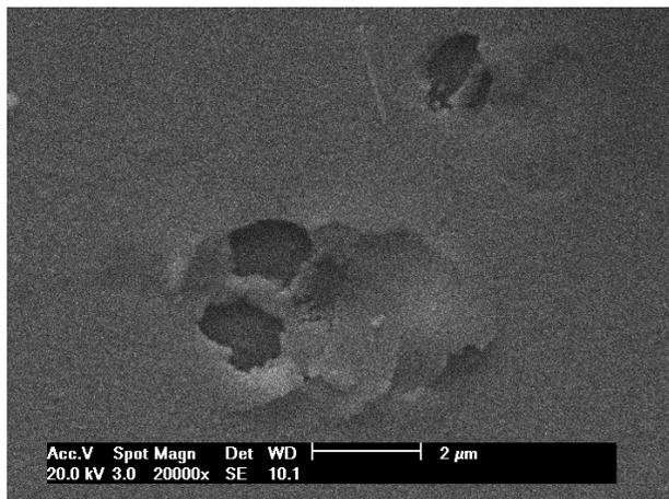
**Figure 6.** SEM of flexible electrochromic device after applying voltage.
