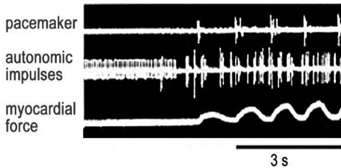
Figure 8. Simultaneous electro-physiological recording: Heart (pacemaker), cardio-regulatory nerve (autonomic impulses), and mechanical transducer (myocardial force, peak=approximately 1mg). An increase of a nerve activity completely stops heartbeat. The smallest spikes in amplitude are the cardio-inhibitory impulses. The other two, the cardio-acceleratory impulses. Specimen, hermit crab ( Aniculus aniculus , modified from Yazawa and Kuwasawa, 1992 [6]).
