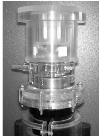
Fig. 1: Concavo-convex Couette flow system.
