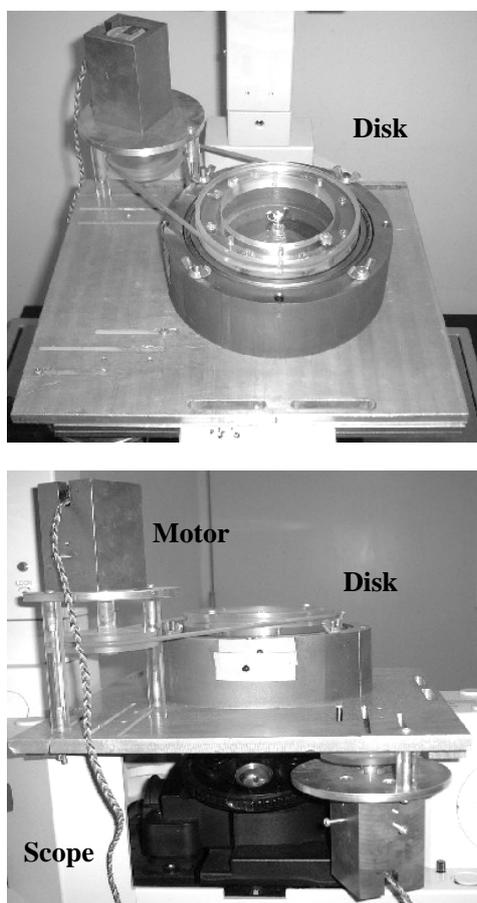
**Fig. 3:** Rheological Couette flow system of counter-rotating parallel disks.
