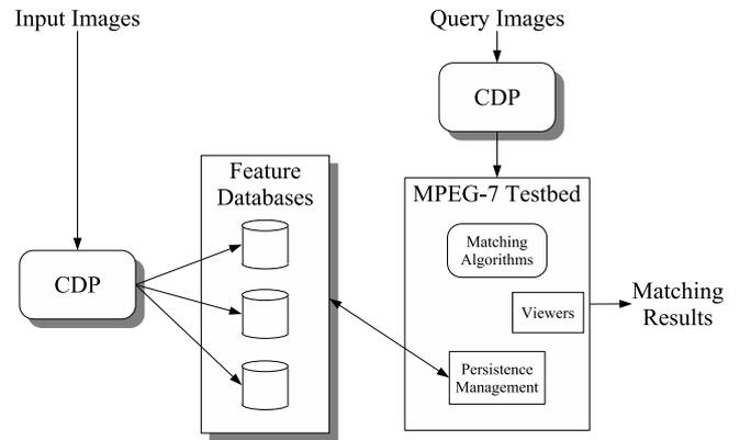
Fig. 5. Integration of CDP and Testbed
