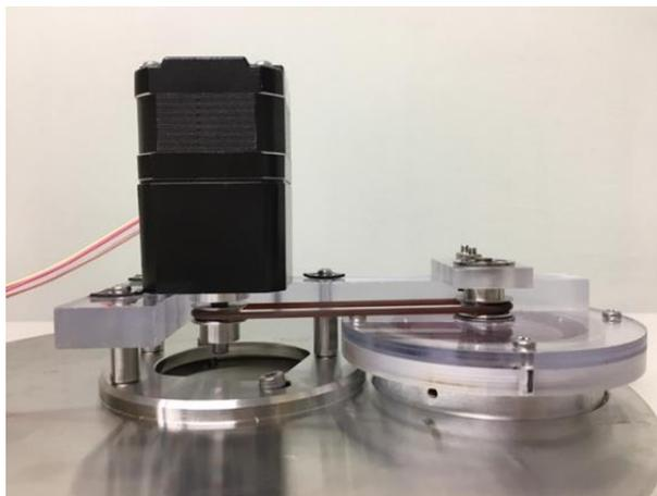
Fig. 2: Manufactured Couette flow device: cross section (upper), and appearance (lower).
