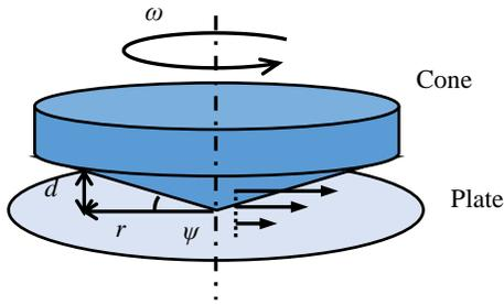
Fig. 1: Couette flow between rotating cone and stationary plate.
