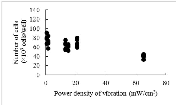
**Fig. 8C:** Number of Hepa1-6 vs. power density of vibration [mW/cm<sup>2</sup>].
