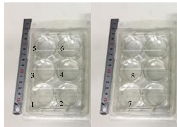
**Fig. 1:** Well number. Piezoelectric element was attached at No. 1. No. 7 and No. 8 are for control.
