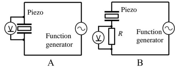
**Fig. 4:** Electric circuit. During stimulation to cell culture (A), Measurement with resistance (B).
