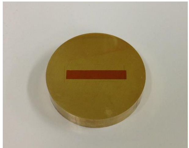
Fig. 4: Mold for upper plate of flow channel.
